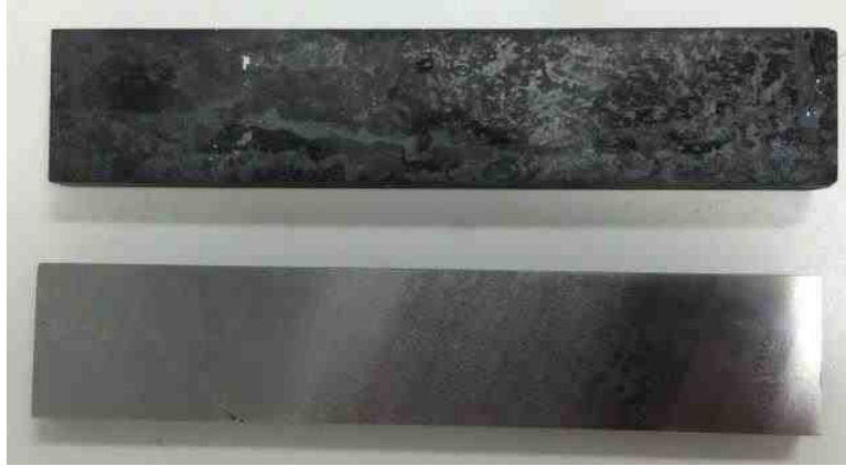
Figure 4. Top:Specimen after heat treatment, Bottom:Specimen after surface preparation
