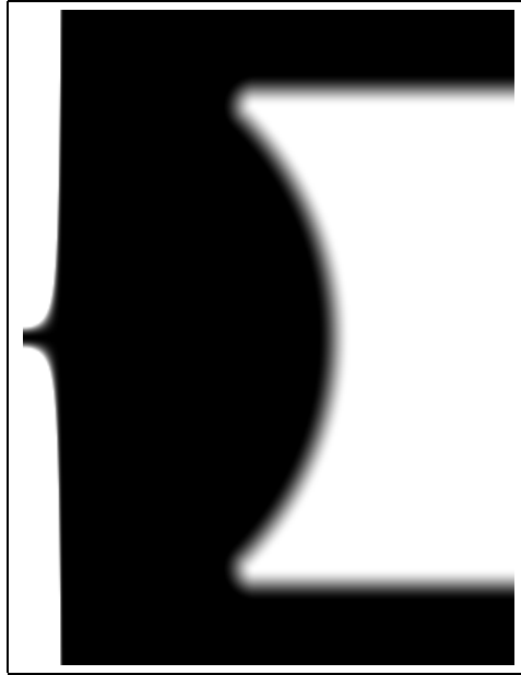
Figure 3.11: This grey-scale image shows the potential used for the resonant cavity in §3.2. The QPC potential is of the same form that we have been considering so far. The mirror part is defined in the following way. First, find the arc desired (here, 90 degrees of arc with the center of curvature at the QPC). Any region to the right of this arc will be held at some given potential higher than the energy of the electrons coming into the resonator. We then sweep a quartic curve around the edge of this region to make the soft wall; the quartic is chosen to match the values and derivatives of the potentials on either side of the soft wall.
