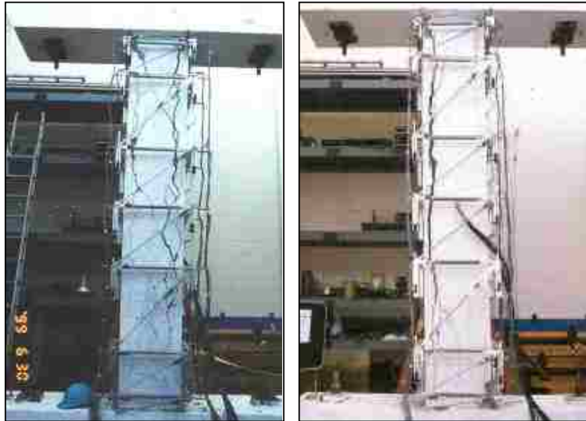
Figures 3.74 and 3.75 Longitudinal cracking on side faces: experimental damage (Sezen 2002)
