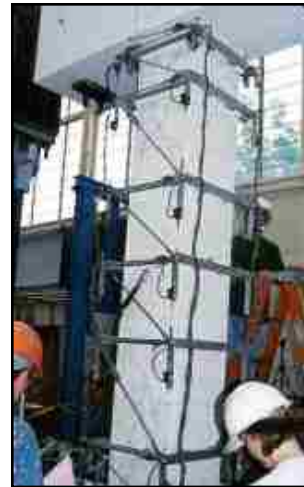
Figure 3.23 (S1 & S2) Flexural and Shear Cracking
