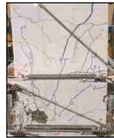
Figures 3.29 and 3.30 (S1 & S2) Flexural and Shear Cracking
