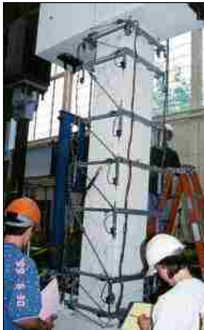
Figure 3.57 Flexural cracking and longitudinal cracking: experimental damage (Sezen 2002)
