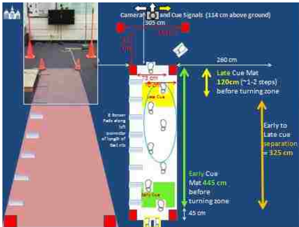
Figure 8. Photo of the Turning Zone with a schematic drawing of the larger lab set-up. Note the “bottle-neck” created by the cones and Gaitrite sensor pad at the entrance to the turn-zone which was spatially confined to a width of about 70 cm (28”) at the level of the feet.
