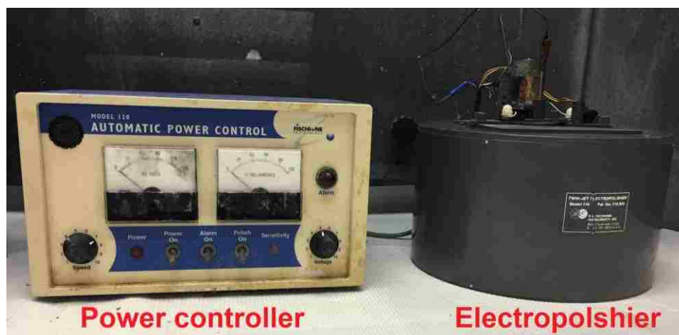
Figure 3.6. The Fischione twin-jet electropolisher employed for making TEM specimens.
