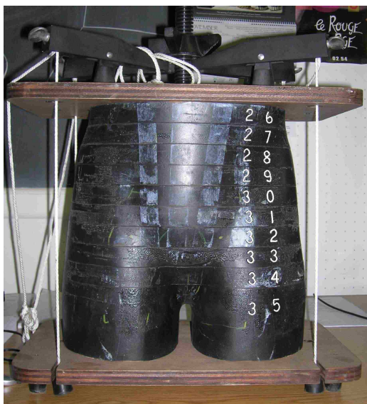
Figure 1.8: The Rando phantom anterior in its holding brace. The slice numbers are colored for better visibility.
