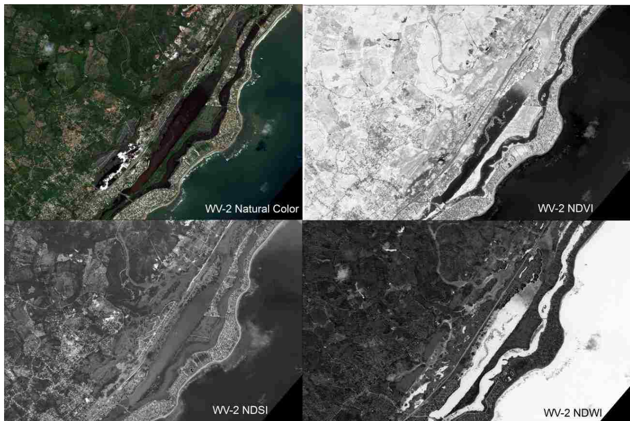
Figure 6.11. WorldView-2 Natural Color Composite and Gray Scale Composite for Vegetation Indices - From top left to bottom right: Natural color composite of WV-2 imagery. Gray scale composite for the vegetation indices: Normalized difference vegetation index (NDVI), Normalized difference soil index (NDSI), and Normalized difference water index (NDWI).
