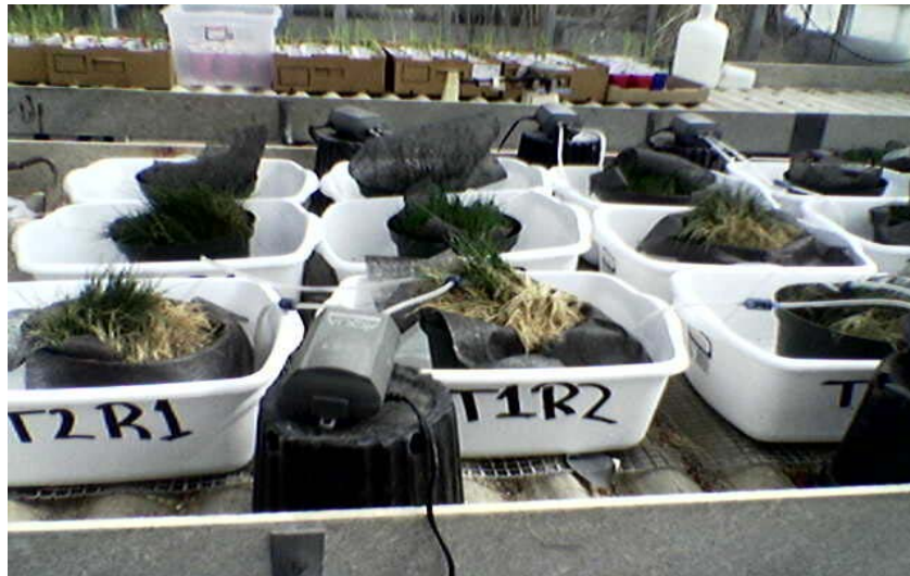
Figure 6: Small scale hydroponic study experimental set up for ryegrass ( Lolium perenne ). Twelve plastic pans contained two liters of hydroponic solution and one ½ gallon plastic pot of seeded ryegrass. The plastic pans were arranged into a randomized complete design with three arsenic treatment levels (0, 1800, and 2500 mg/L) and four replications of each treatment level
