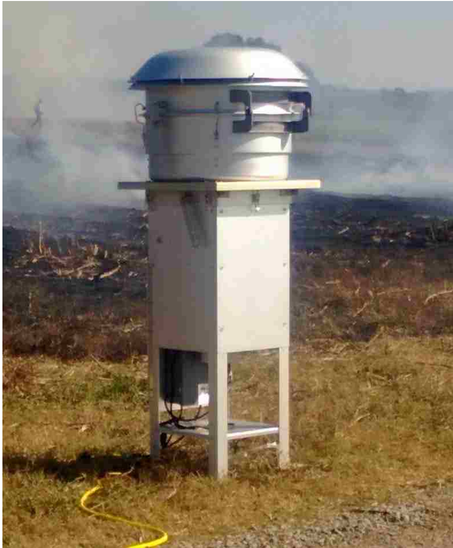
Fig 4.1. High volume air sampler (HVAS) installed in the field for collecting particles from burning sugarcane residues
