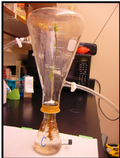
Figure 24. Reactor Used to Determine the Fate of Cumene and 4-Cumylphenol in a Black Willow Cutting
