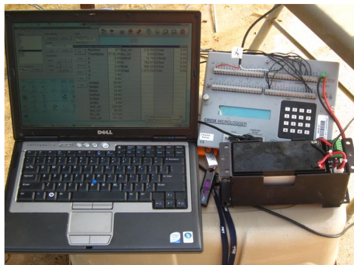
Figure 2. Campbell Scientific CR23X datalogger and PC computer system used to monitor leaching fraction during leaching simulation experiment in 2012.
