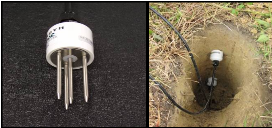
Figure 4.6. Stevens Vital soil moisture, temperature, and salinity sensor with depiction of typical installation in excavation wall at 20 cm and 50 cm depths. Cables were buried in trenches.
