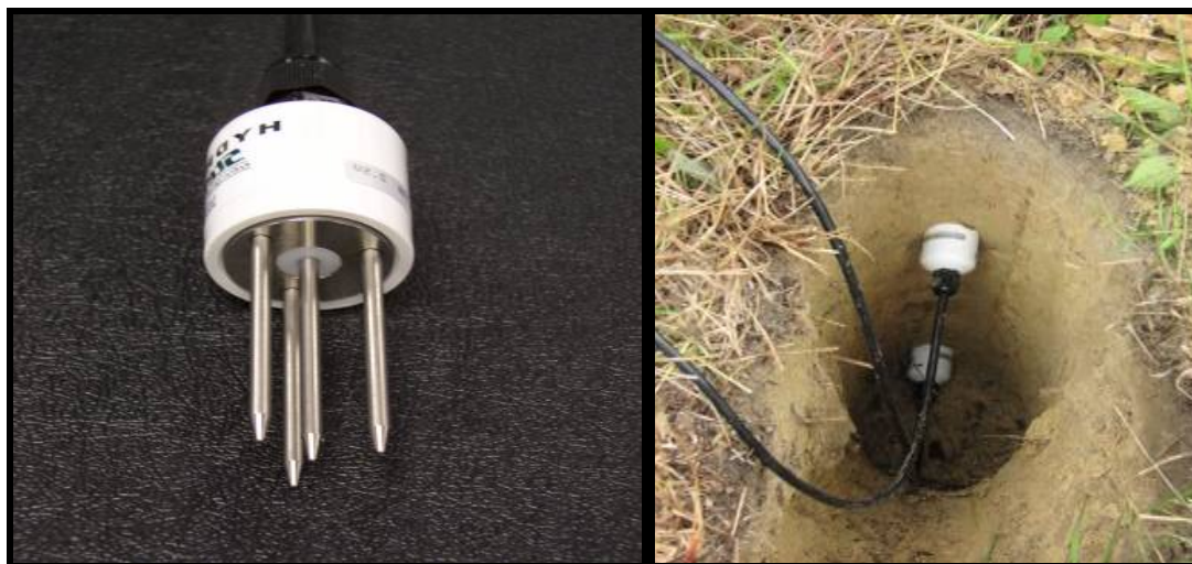
Figure 3.7. Stevens Vital soil moisture, temperature, and salinity sensor with depiction of typical installation in excavation wall at 20 cm and 50 cm depths. Cables were buried in trenches.
