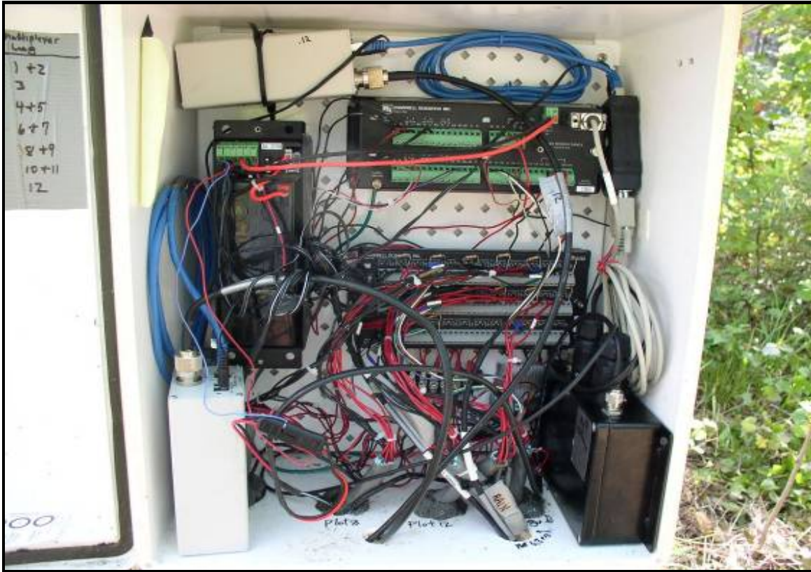
Figure 4.5. Primary site data logging station with Campbell Scientific CR-10X ® datalogger, CSI AM16/32 multiplexer, radio telemetry, satellite uplink, and atmospheric environmental monitoring equipment.
