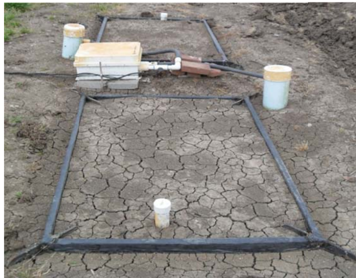
Figure 3.2 Weighing lysimeters, viewed from the southeast toward the northwest, LSU AgCenter Northeast Research Station, Saint Joseph, LA.
