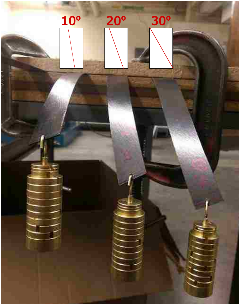
Figure 2.2: Bend-twist coupled spars of varying fiber angle under equal load.
