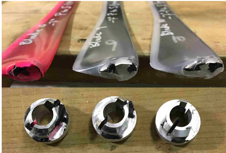
Figure 7.9: Pitch to stall blade failure between blades (top) and root connection (bottom).
