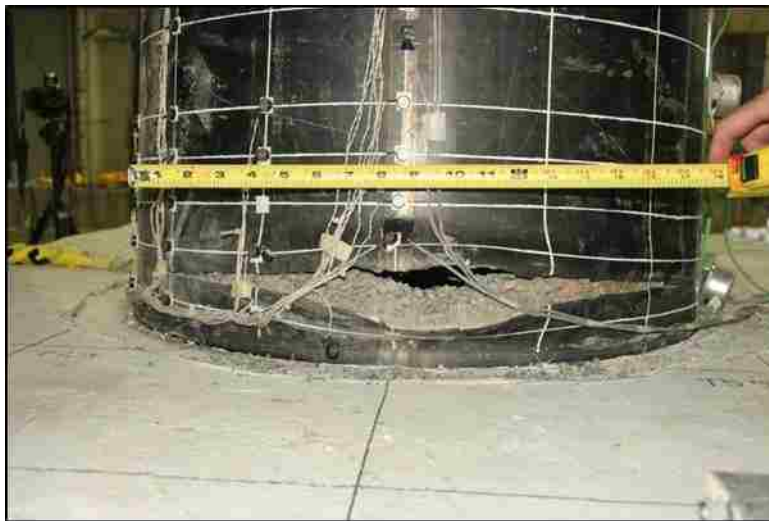
Figure 5.71: EMB96 South tear propagation at 9.15% drift North
