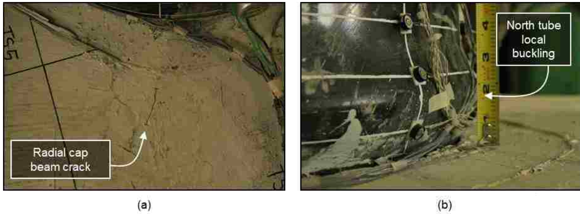
Figure 5.67: EMB96 (a) South cap beam cracking and (b) North column buckling after 13 th load set
