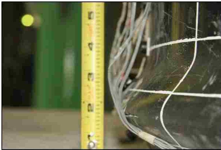
Figure 5.69: EMB96 Initiation of South tube tearing
