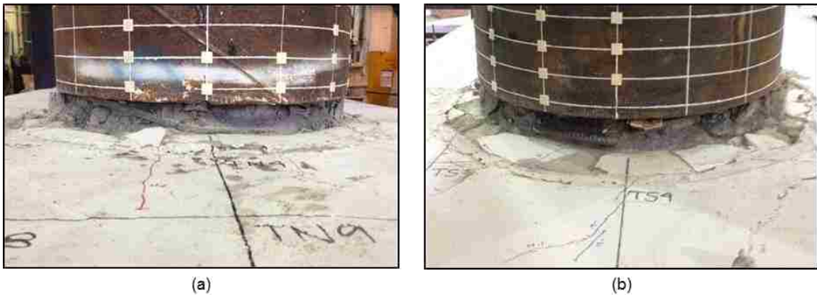
Figure 5.61: WRC(a) North and (b) South side of specimen after removal of spalled grout
