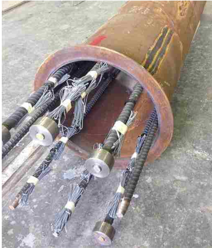
Figure 4.11: Specimen WRC annular ring and reinforcing bars
