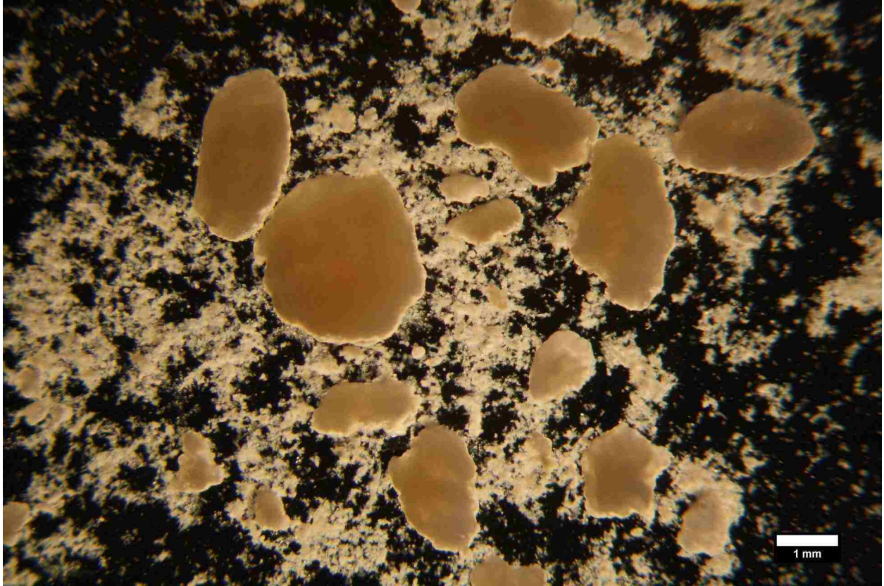
Figure C7. Mainstream reactor mixed liquor suspended solids on the third day of the bioaugmentation period (6x magnification and 1mm scale bar).
