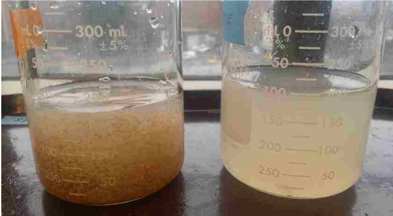
Figure C8. Mainstream reactor mixed granular (left) and flocculent (right) solids fractions after sieving protocol.
