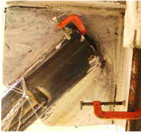
Figure 4.41: GP yielding at 1.7% drift (Y1).
