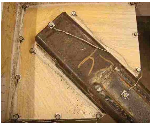
Figure 4.63: Mid-span GP initial yielding at 0.4% drift (Y1).
