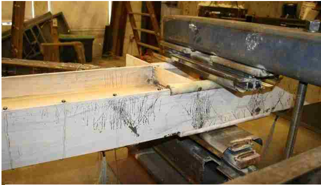
Figure 4.72: Beam OF yielding at 1.9% drift (Y1-OF).
