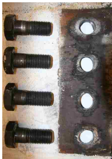
Figure 4.57: N beam web bolt hole elongation.
