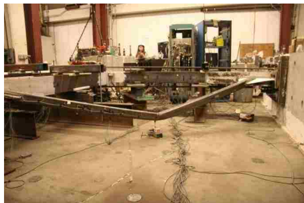
Figure 4.53: N brace buckling at 3.3% drift (B3-PH).
