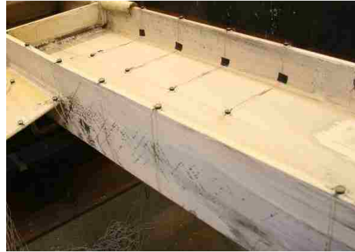
Figure 4.73: Beam IF yielding at 1.9% drift (Y1-OF).
