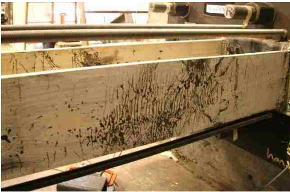
Figure 4.43: S col. moderate yielding at 1.9% drift (Y1-OF/IF).
