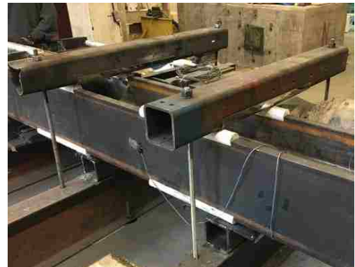
Figure 3.16: Installed out-of-plane restraints.
