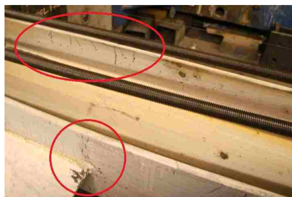
Figure 4.40: S col. initial yielding at +1.4\% drift (Y1-OF).
