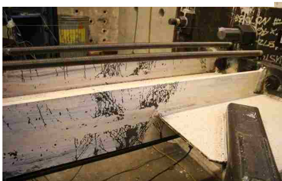
Figure 4.70: N col. moderate yielding at 1.9% drift (Y2-PH).
