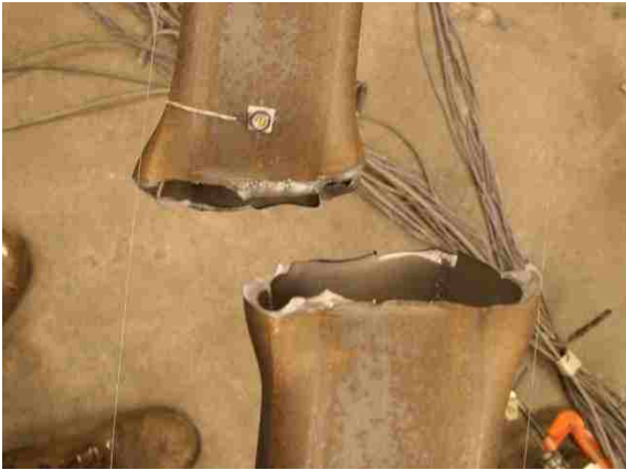
Figure 4.88: N brace fracture at -3.6% drift (B4-BF).
