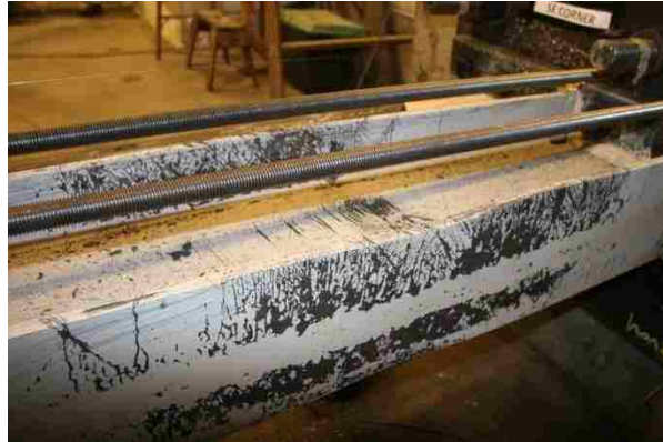
Figure 4.77: S col. severe yielding at 2.8% drift (Y3-PH).
