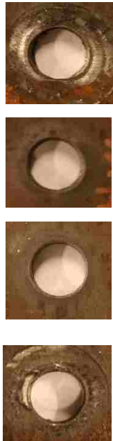
Figure 4.56: S beam web bolt hole elongation.
