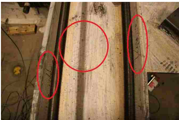
Figure 4.11: N col. initial yielding at +1.4\% drift (Y1).
