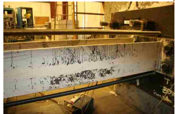
Figure 4.71: S col. moderate yielding at 1.9% drift (Y2-PH).
