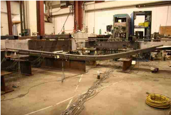
Figure 4.9: N brace buckling at +1.1\% drift (B2).
