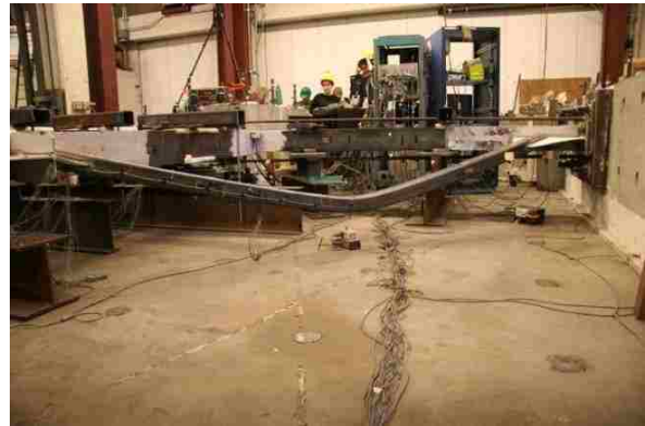
Figure 4.46: Brace buckling at 2.5% drift (B1).
