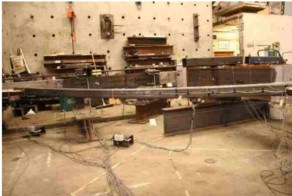
Figure 4.6: S brace buckling at -0.28% drift (B1).
