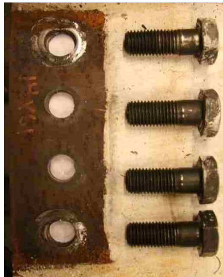
Figure 4.56: S beam web bolt hole elongation.
