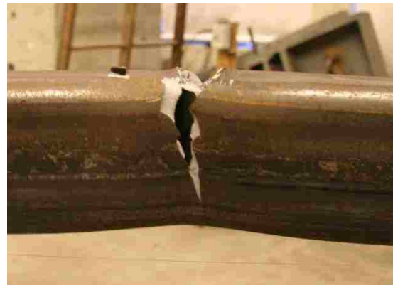
Figure 4.85: S brace \frac{3}{4} tear at 3.6% drift (B3-BT).
