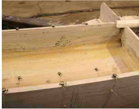
Figure 4.42: Beam IF initial yielding at 1.9% drift (Y1-IF).
