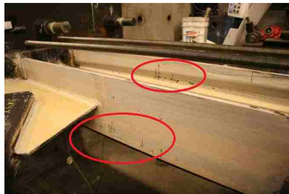
Figure 4.69: S col. initial yielding at 1.4% drift (Y1-OF/IF).
