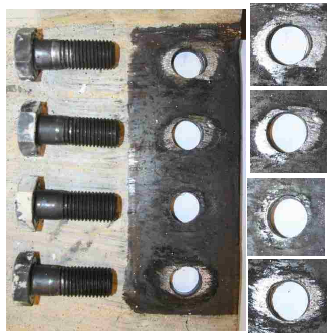
Figure 4.91: N beam web bolt hole elongation.
