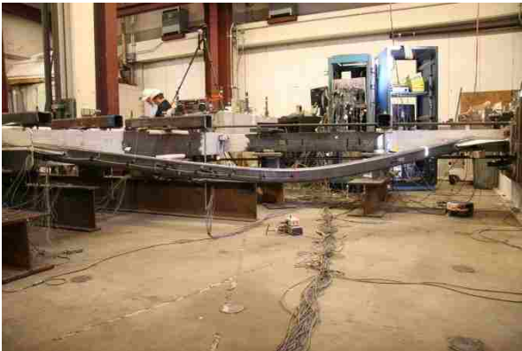
Figure 4.37: N brace buckling at +1.1\% drift (B1).
