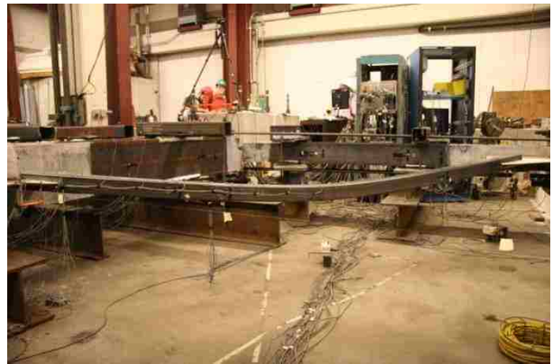
Figure 4.7: N brace buckling at +0.7% drift (B1).
