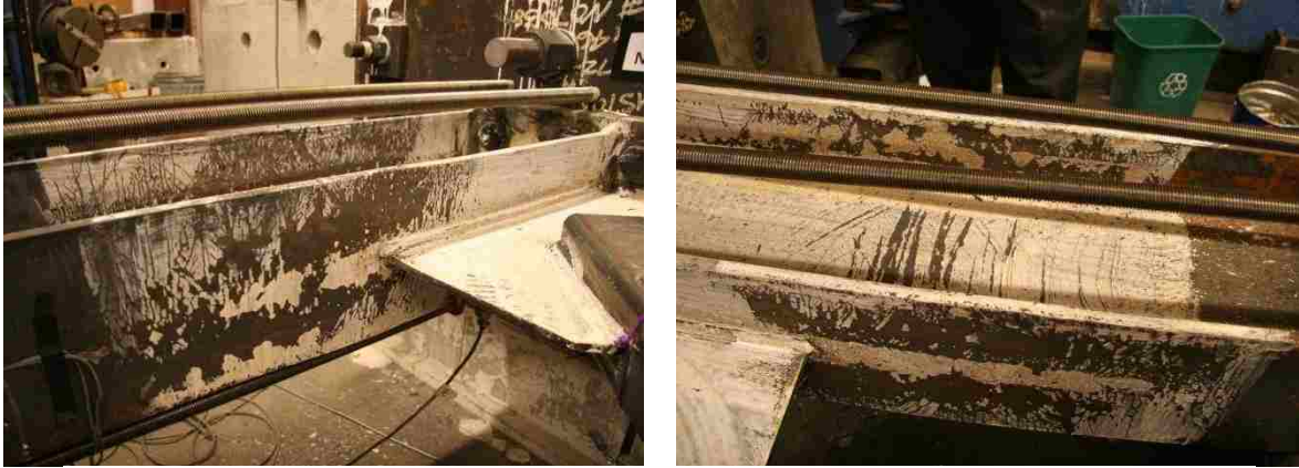
Figure 4.22: Severe yielding in N col. (left) and S col. (right) at 2.76% drift (Y3-PH).
