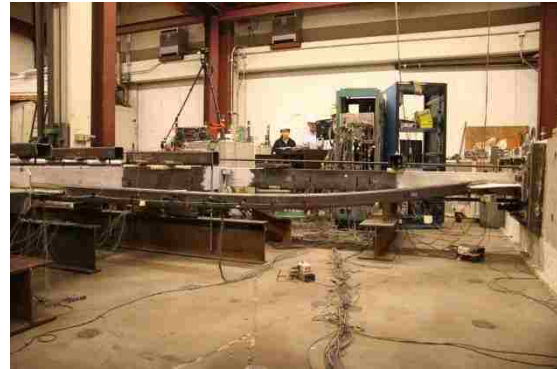
Figure 4.34: N brace buckling at 0.41% drift (Y1).
