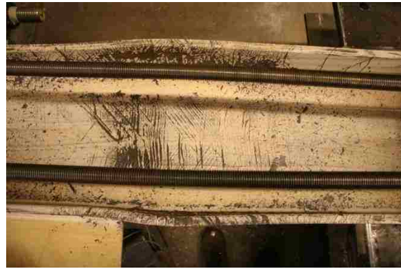
Figure 4.79: S col. moderate local buckling 3.0% drift (LB2-OF/IF).
