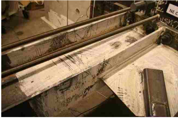
Figure 4.13: N col. moderate yielding at +1.9% drift (Y2-PH).
