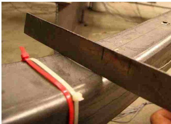
Figure 4.15: S brace initial cupping at -1.9% drift (B3-PH).
