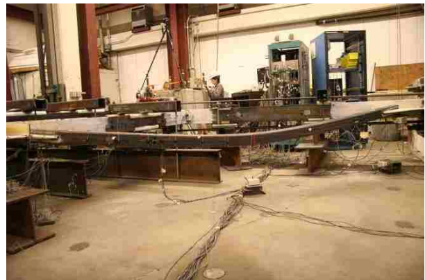
Figure 4.62: N brace buckling at 0.7% drift (B1).
