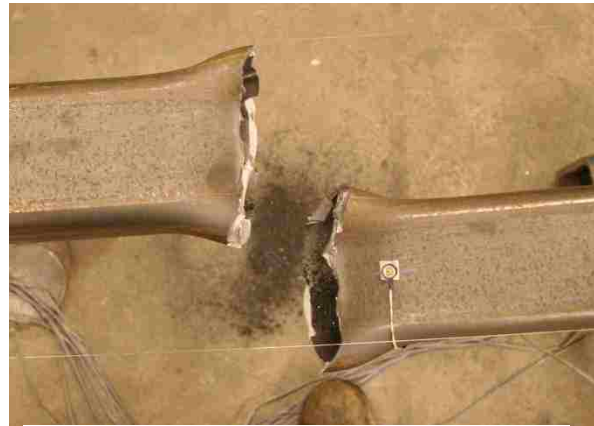
Figure 4.89: S brace fracture at +3.6% drift (B4-BF).
