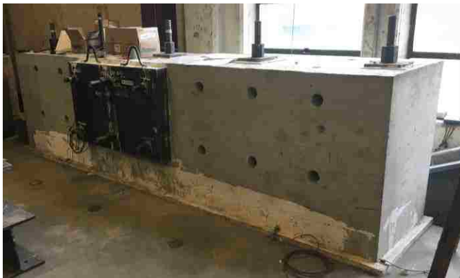
Figure 3.2: Reaction block used for N column anchorage.
