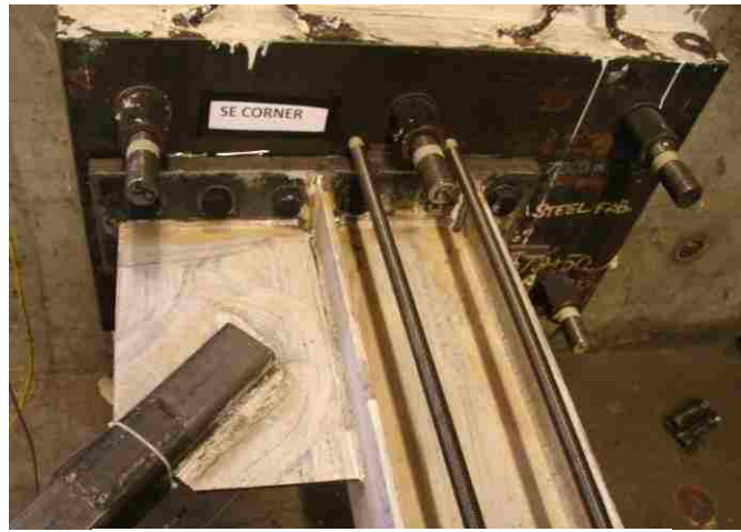
Figure 3.8: Base plate attached to interface plate.
