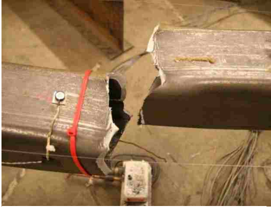
Figure 4.54: N brace fracture at -3.3% drift (B4-BF).
