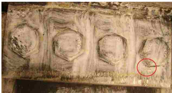
Figure 4.61: S shear tab initial yielding at 0.41% drift (Y1).
