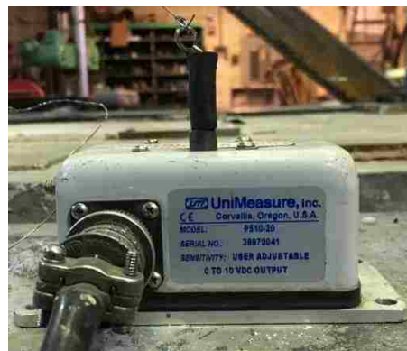
Appendix Figure H.5. UniMeasure ® string potentiometer.
