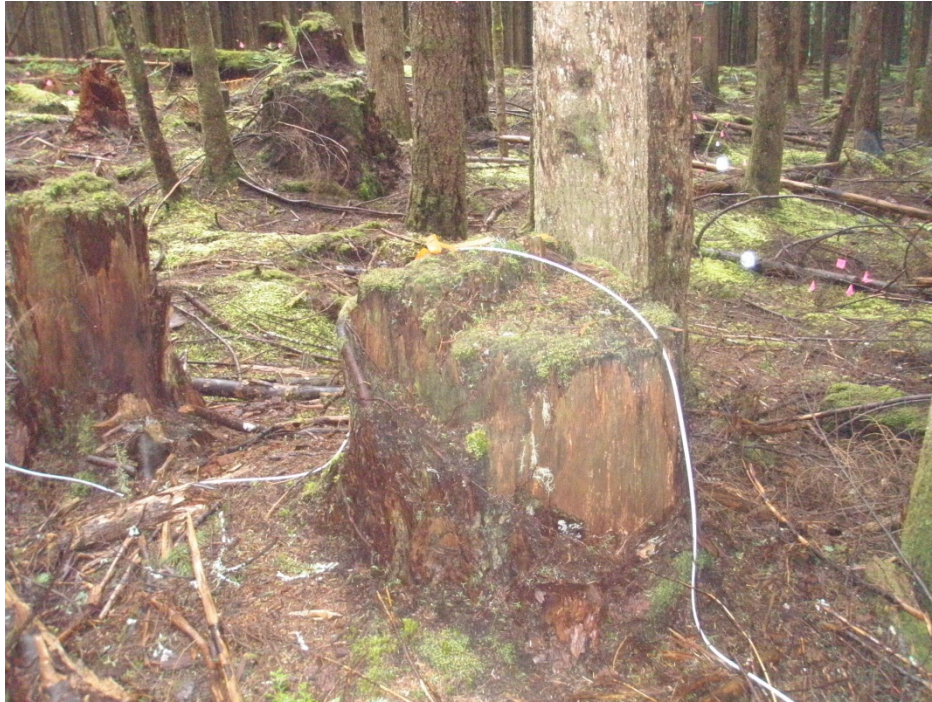
Figure 3.9 Photograph of the fiber-optic cable draped over a large stump, resulting in temperature observations that represents the stump or the adjacent air space rather than the ground temperature.
