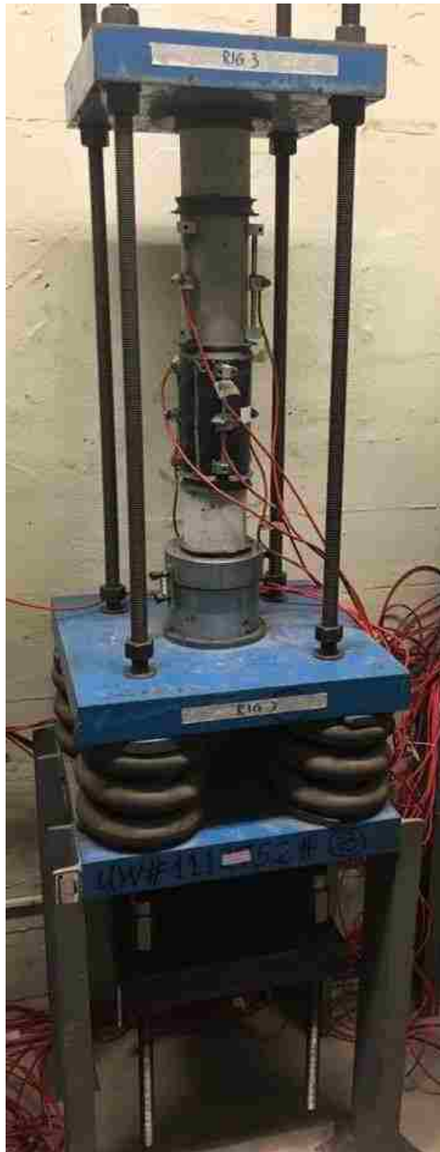
Figure 3.5 A Loaded Creep Rig in the Lab
