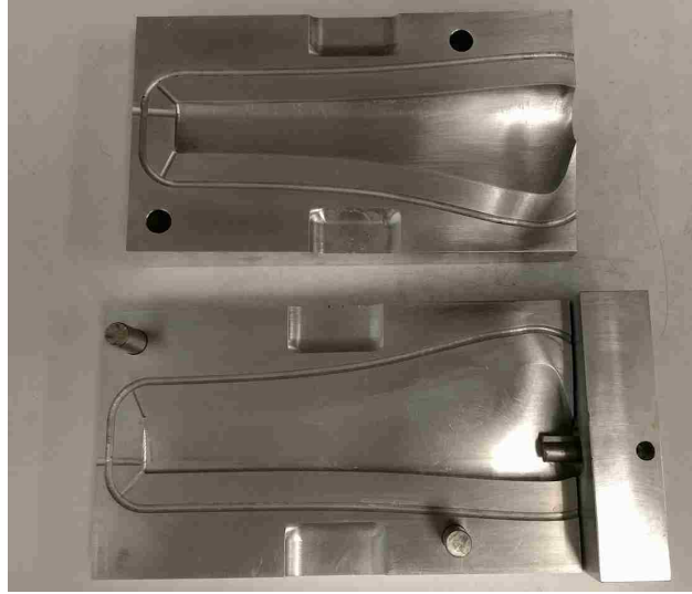
Figure 5.3: Machined aluminum mold of flume-scale blade geometry
