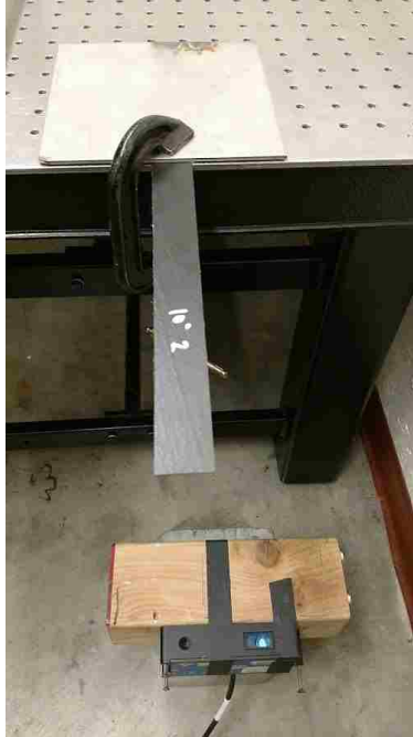
Figure 2.5: Experimental setup for free vibration
