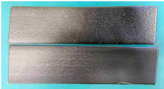
(a) Autoclave-cured laminates used for composite spar
