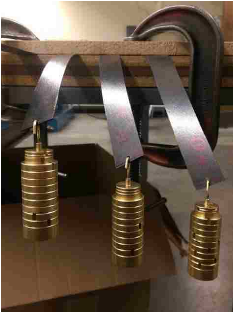
Figure 2.4: Deflection of varied fiber angle ( 10^\circ , 20^\circ , 30^\circ ) beams under identical loading
