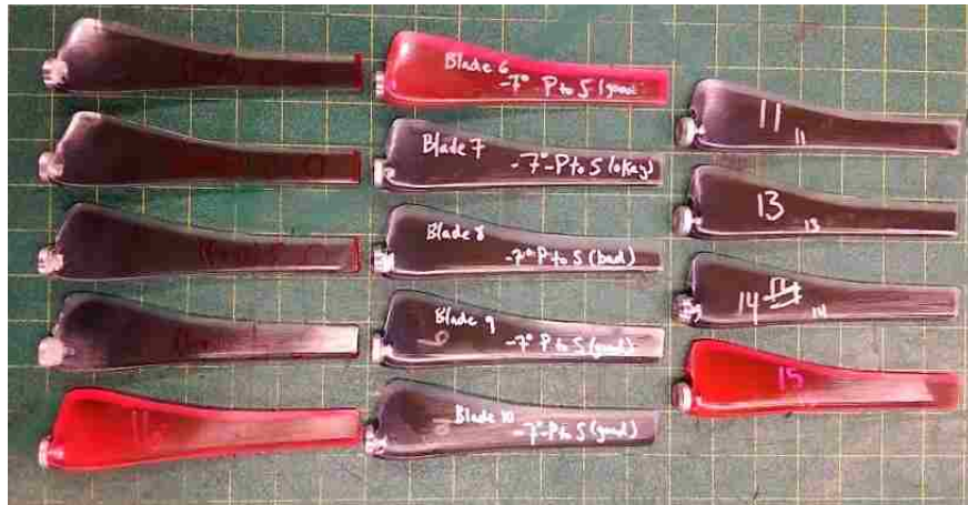
Figure 5.7: Finished blades with flexible urethane poured over the spars
