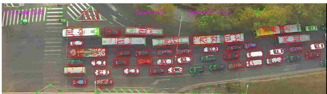
Figure 7-6 Selected sample frames showing the vehicle detection and parameter estimation results in congested condition
