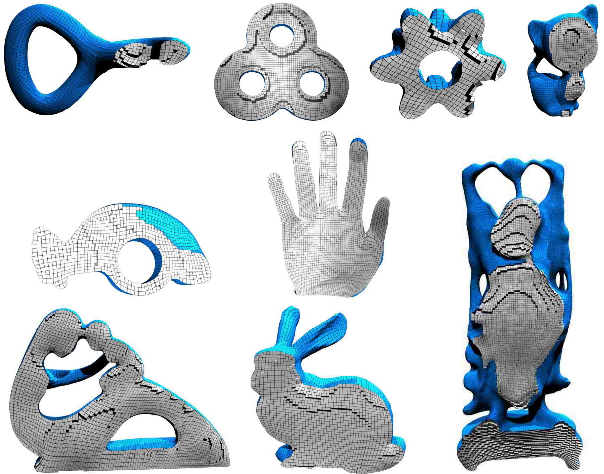
Figure 5.6: Hex Meshing Results for Double Torus, 3-Torus, Bump Torus, Hand, Rocker arm, Kitten, Fertility, Bunny and Buddha.
