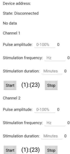
Figure 5.2. Android layout for 2-channel device. The user can set stimulation parameters, read current stimulation parameter settings, and start and stop stimulation.
