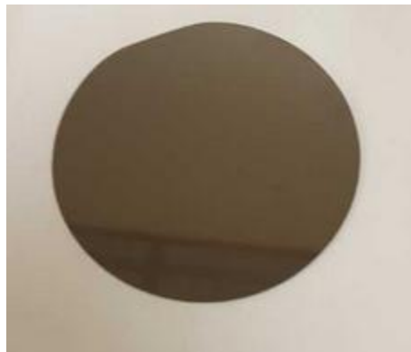
Figure 8.1. Photograph of the \langle 1-0-0 \rangle Silicon wafer
