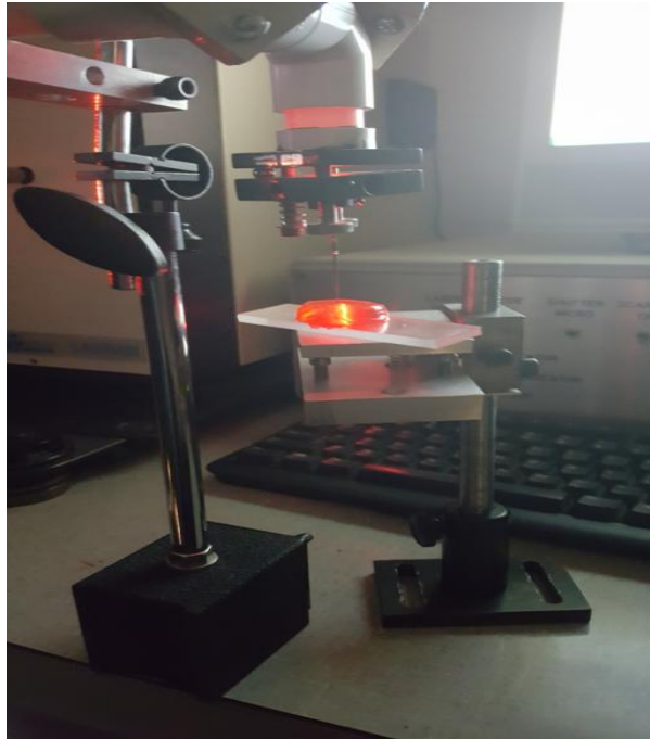
Figure 6.1. Photograph of Probe at end of articulated arm inserted in Gelatin block
