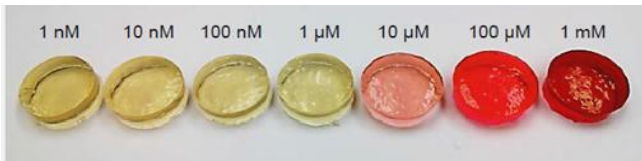
Figure 4.5. Gelatin prepared with different concentrations of R6G solutions varying from 1nM to 1mM for ex vivo like measurements
