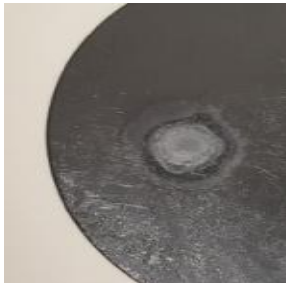
Figure 8.3. Optical image of the Silicon wafer after removing 120 \mu\text{m} using small tube to define the etched area.
