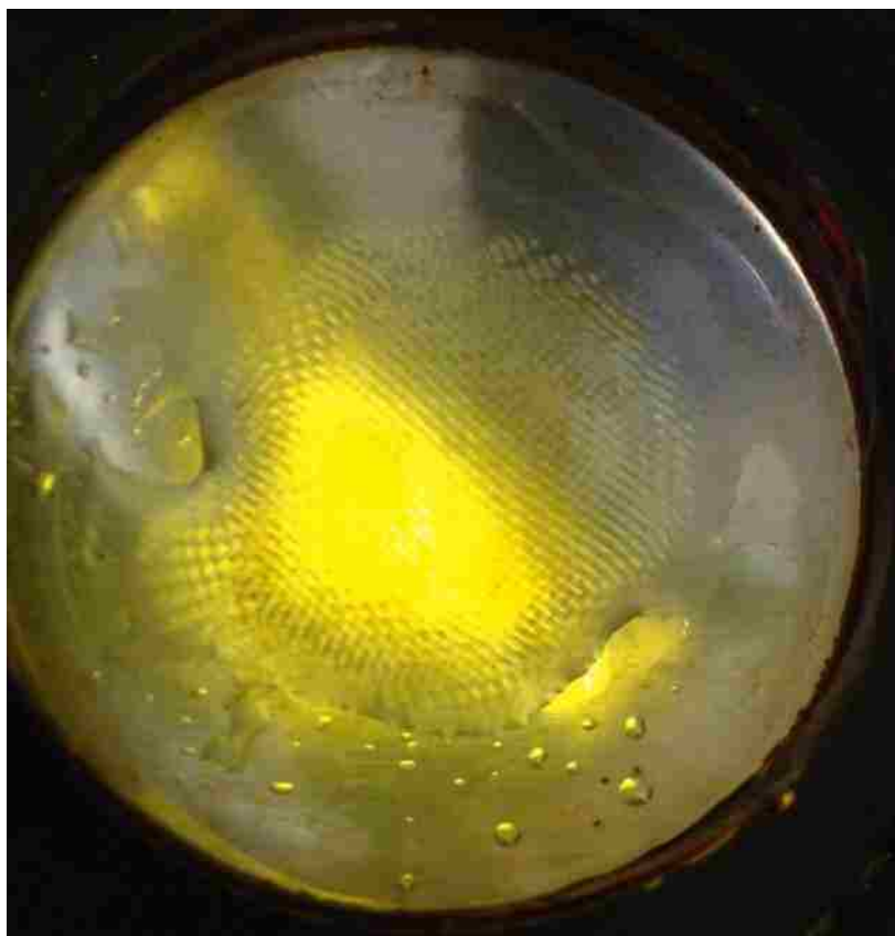
Figure 6-5: Liquid wave patterns on the free surface generated by the sound waves
