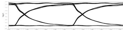
(e). The eye diagram of memory bus when writing data to devices in the single-link mode
