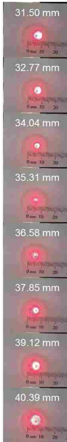
Fig. 5.6 The reflected laser beam from the gold surface makes the best focus with the distance of approximately 35.31 mm between the second lens and the first surface of GRIN lens.
