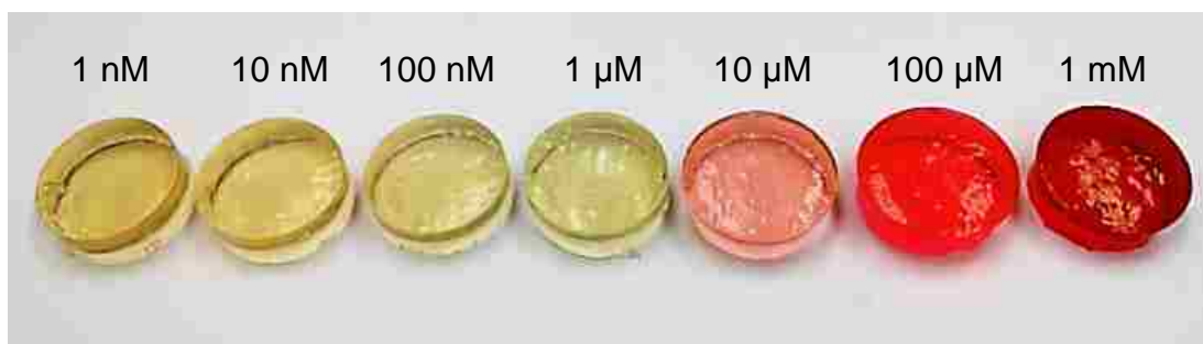
Fig. 4.7 Gelatin with different concentrations of Rhodamine 6G.
