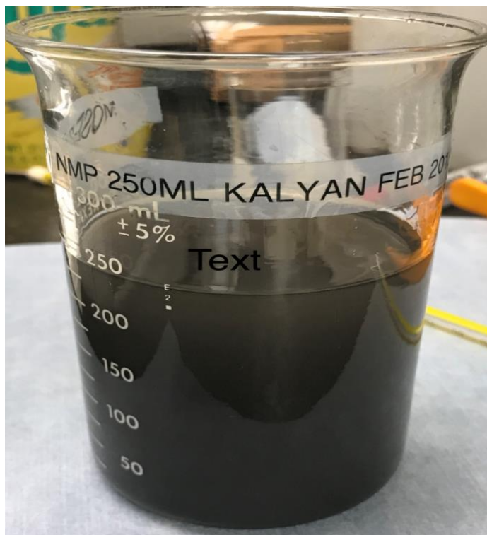
Figure 4.1. Dispersed solution of MoSe 2 in NMP
