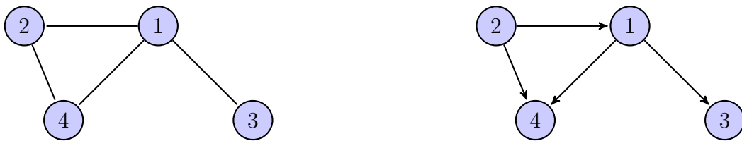
Figure A.1: a) Left: Undirected Graph: \mathcal{V} = \{1, 2, 3, 4\} , \mathcal{E} = \{(1, 2), (1, 3), (1, 4), (2, 4)\} . b) Right: Directed Graph: \mathcal{V} = \{1, 2, 3, 4\} , \mathcal{E} = \{(1, 3), (2, 1), (1, 4), (2, 4)\} .
