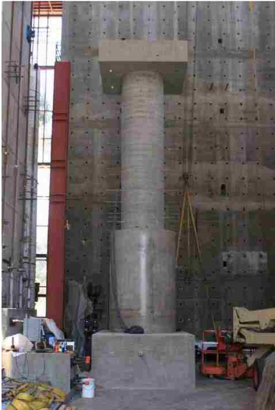
Figure 7-4. Cast-in-place column-shaft connection specimen (Murcia-Delso et al. 2013)
