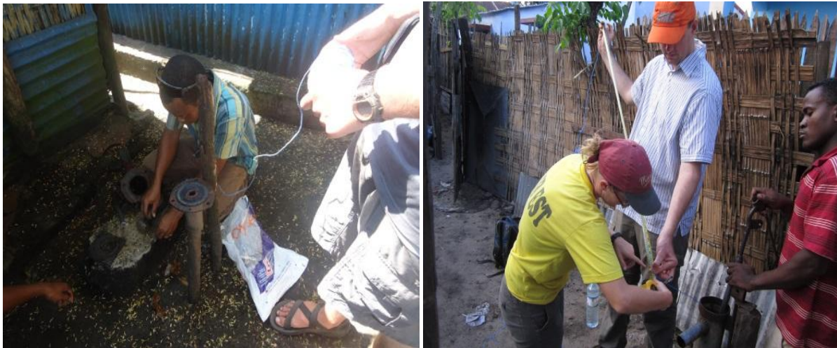
Figure 10: Process used to measure the depth of the wells. (a) Measuring the depth of the well by lowering a string with a weight to the bottom of the well. The local Malagasy technician (pictured on the left) is preparing a replacement weighted leather check valve to be installed after the measurement is complete (picture taken by the author); (b) Measuring the length of the rope (picture taken by D. Brad Akers).
