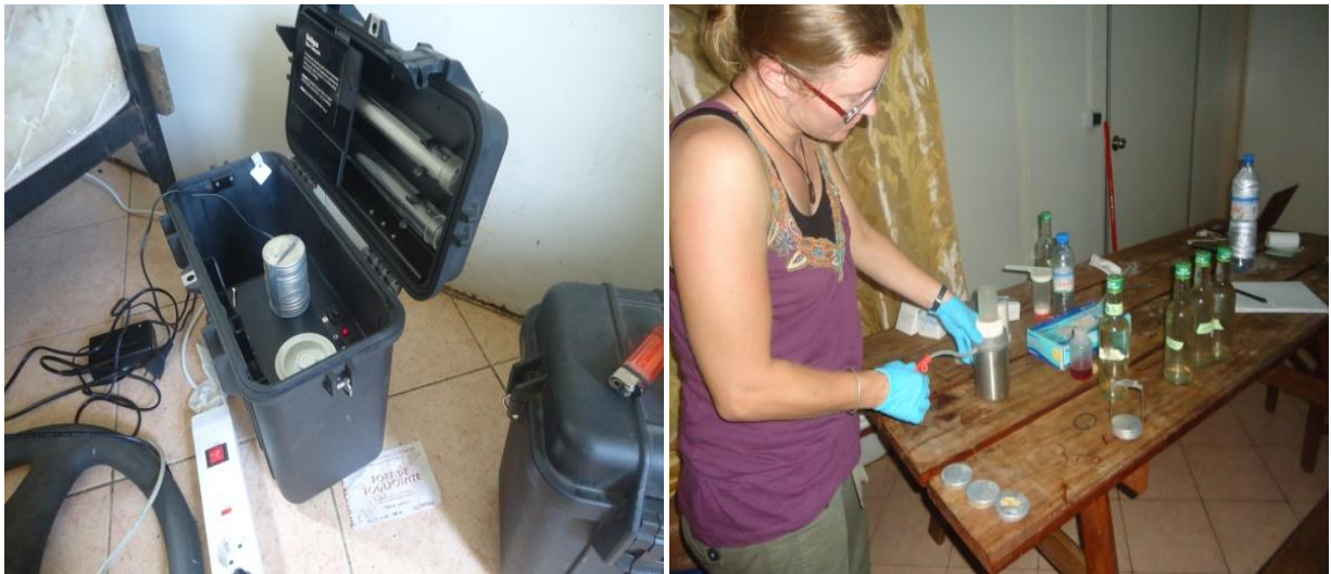
Figure 9: Sample processing equipment. (a) DelAgua incubator portable incubator and metal petri dishes (picture taken by the author); (b) Laboratory set up within the house in Tamateve. Photo is showing the handheld filter apparatus, sample collection containers, metal petri dishes and absorbent pads (picture taken by Brad Akers).
