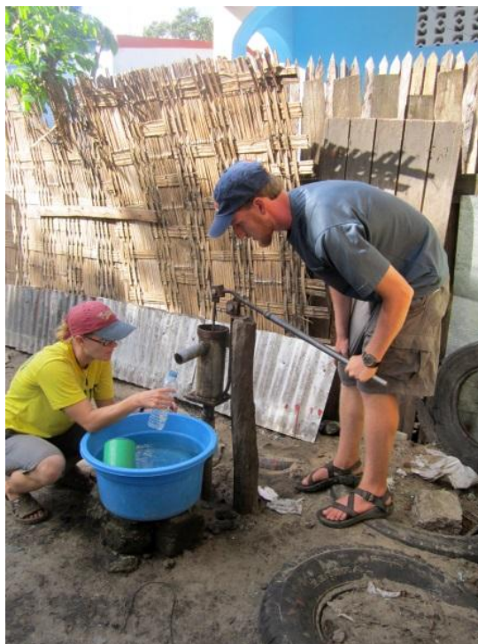
Figure 8: Collecting a sample to be used for the analysis of thermotolerant coliforms (picture taken by Michael MacCarthy).
