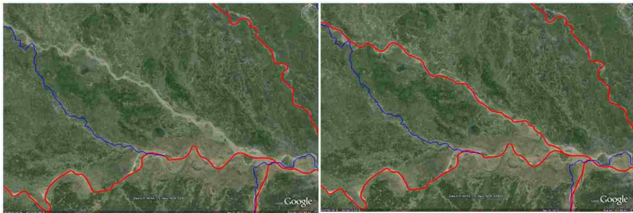
Figure 2.13 : Comparison between SRTM DEM generated river network (Blue color) and newly (corrected) digitized river network (Red color)
