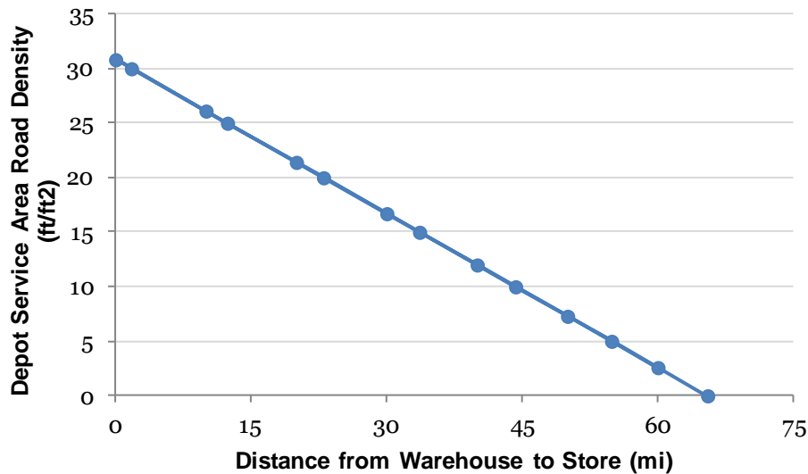
Figure 12: Sensitivity Analysis Threshold Comparing Influences on CO 2 Emissions between Passenger Vehicles and Warehouse Delivery Goods Movement Schemes
