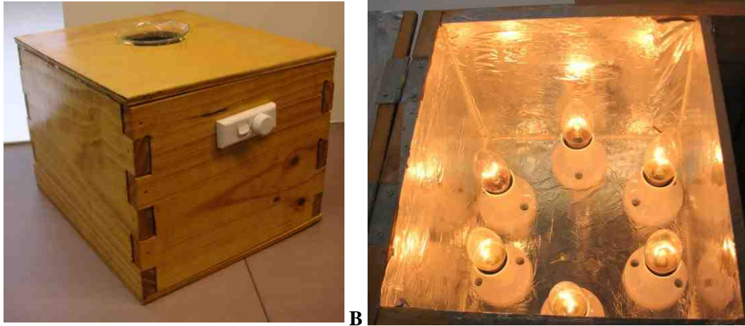
Figure 2.23. (A) External photograph of the custom made heat bath, indicating the white dimmer switch and the placement of the saline containing vessel on top of the pine box. (B) Inside the heat bath, showing aluminium foil layered on pine walls and six globes which would surround the clear glass saline containing vessel at 60° separations.
