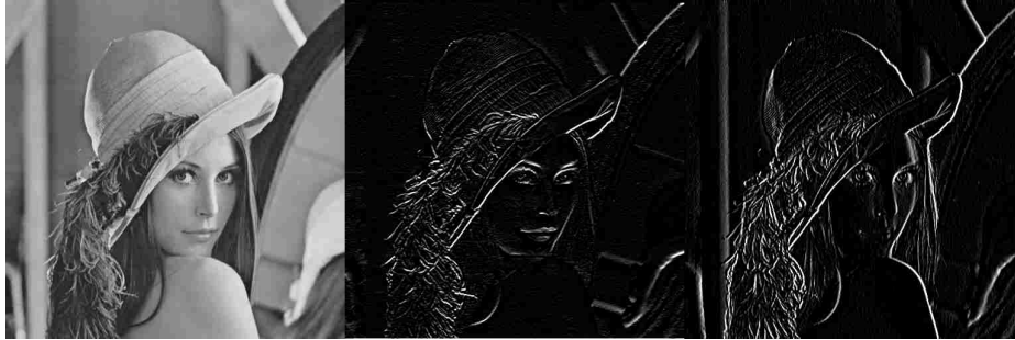
Figure 3.17: lena.png (left), horizontal Sobel filtered (middle), and vertical Sobel filtered (right).
