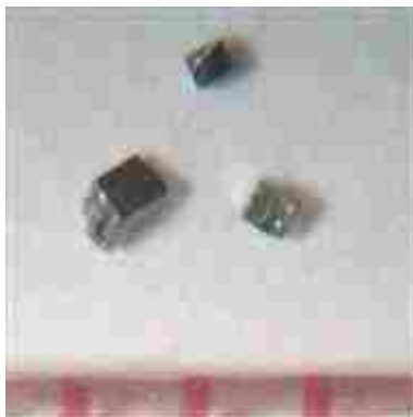
Figure 2.1. Three single crystals of \text{ErCr}_{0.14}\text{Ga}_3 with a mm scale.
