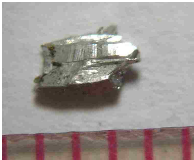
Figure 7.1. A single crystal of Yb 2 Pd 3 Ga 9 on a mm scale.
