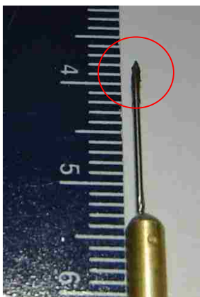
Figure E.2. The sample holder used for temperature-dependent X-ray diffraction experiments.
