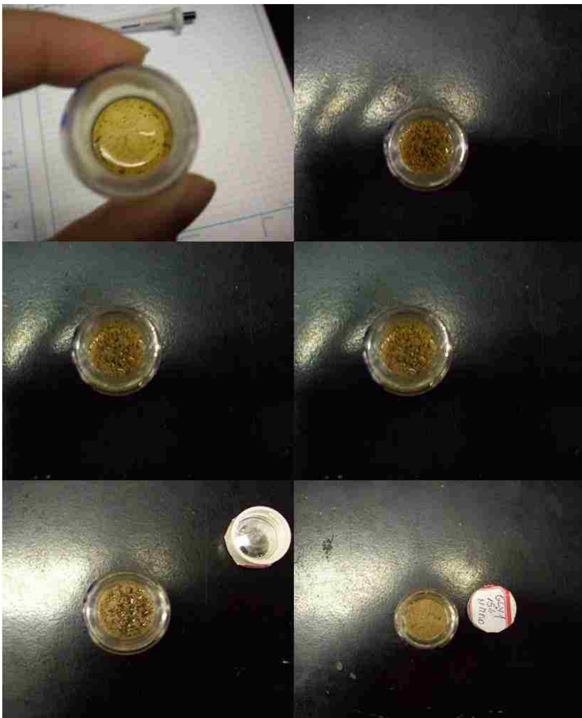
Figure 4.4 Nucleation and growth exhibited by a 15% solution of glylon-6,6 in NMMO x H 2 O. The diameter of vial was 20mm.
