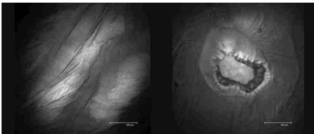
Figure 4.11 Confocal images of fibrils (left) and nucleation point (right) for a 15% solution of gly-6,6 in NMMO monohydrate. The sample was placed between two glass covers separated by an O-ring. The scale bar is 300 \mu\text{m} .
