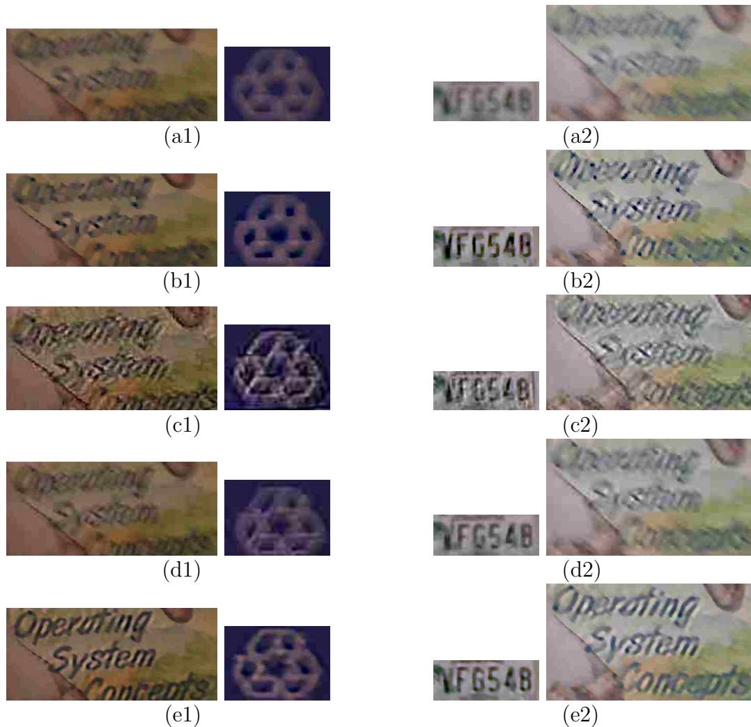
FIGURE 4.5. Comparison of state-of-the-art blind image deblurring algorithms (Zoomed-in regions). (a1) and (a2) Two original space-varying blurred images; (b1) and (b2) Deblurred images using Cho's method [37]; (c1) and (c2) Deblurred images using Shan's method [34]; (d1) and (d2) Deblurred images using Xu's [45] method; (e1) and (e2) Deblurred images using my method;
