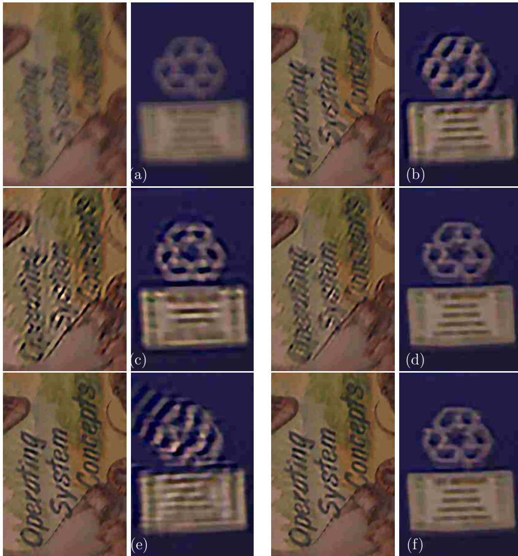
FIGURE 4.3. Zoomed-in regions. (a) Input image, same as in Figure 4.2(a); (b) Deblurred image, given in Figure 4.2(i); (c) Deblurred image, given in Figure 4.2(j); (d) Deblurred image, given in Figure 4.2(k); (e) Deblurred image, given in Figure 4.2(l); (f) Final deblurred image given in Figure 4.2(m).
