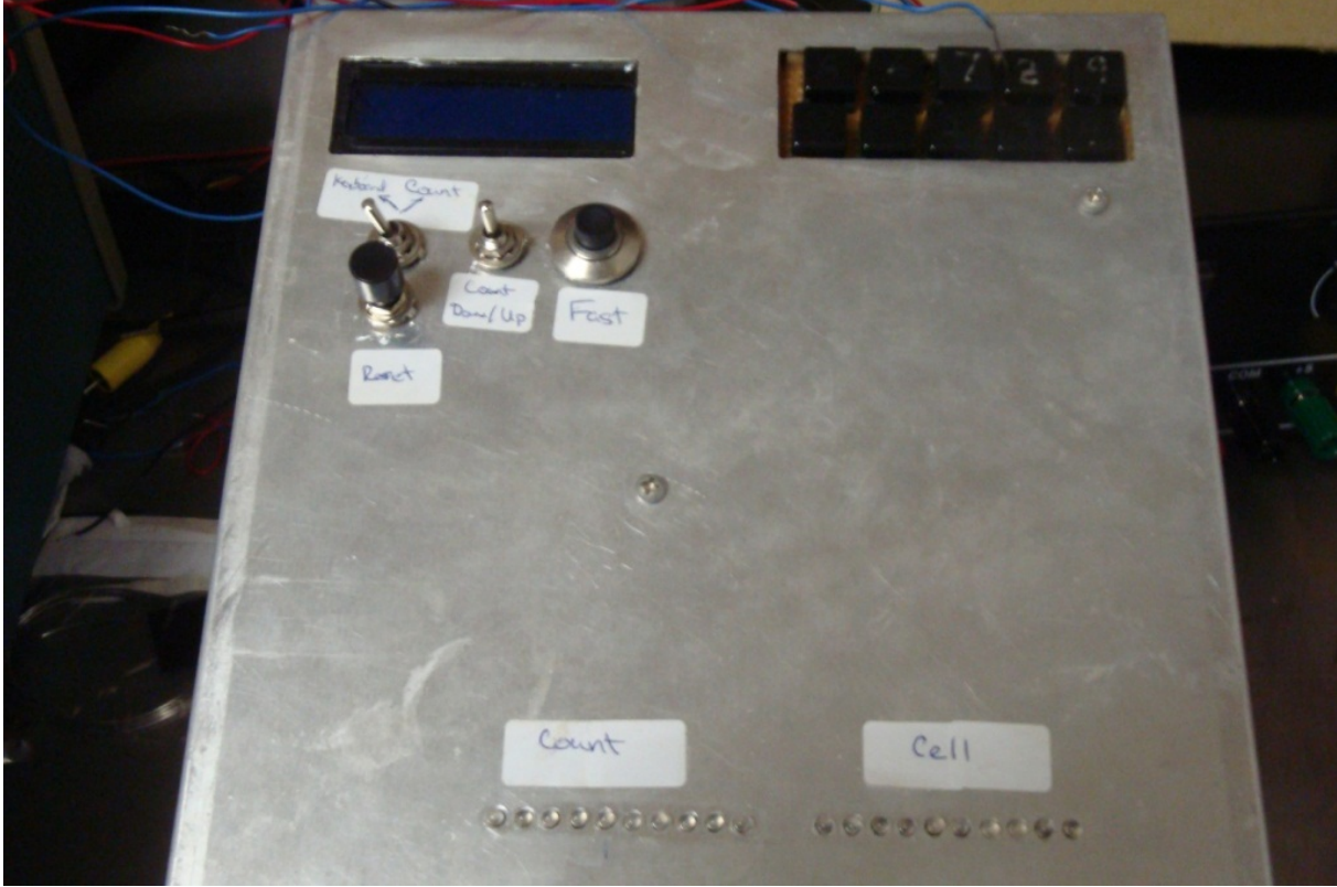
Figure 7-10: The digital system used to control the optical system. The electronics are assembled into an enclosure for protection and organization.
