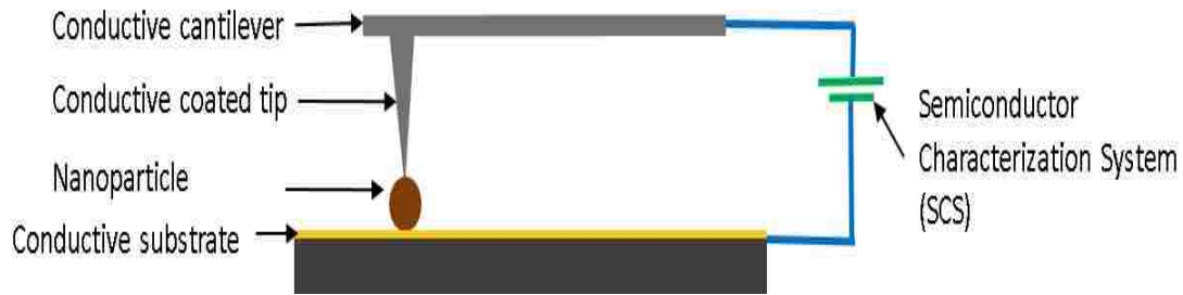
Figure 9: Schematic a of conductive probe AFM system
