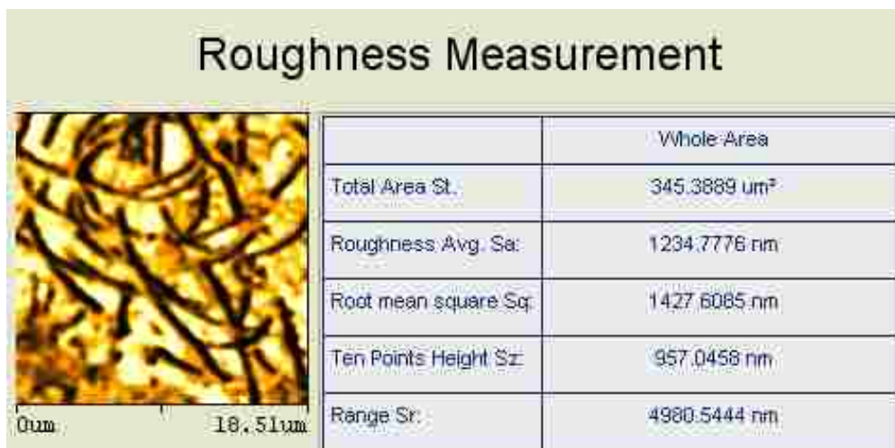
Figure 32:Roughness analysis of zein fibers on glass substrate (18.51X18.51 µm 2 area)
