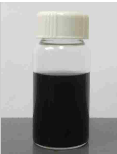
Figure 4-1: Dispersed CNT solution obtained after bath sonication of the acid-refluxed CNTs used for EPD experiments.
