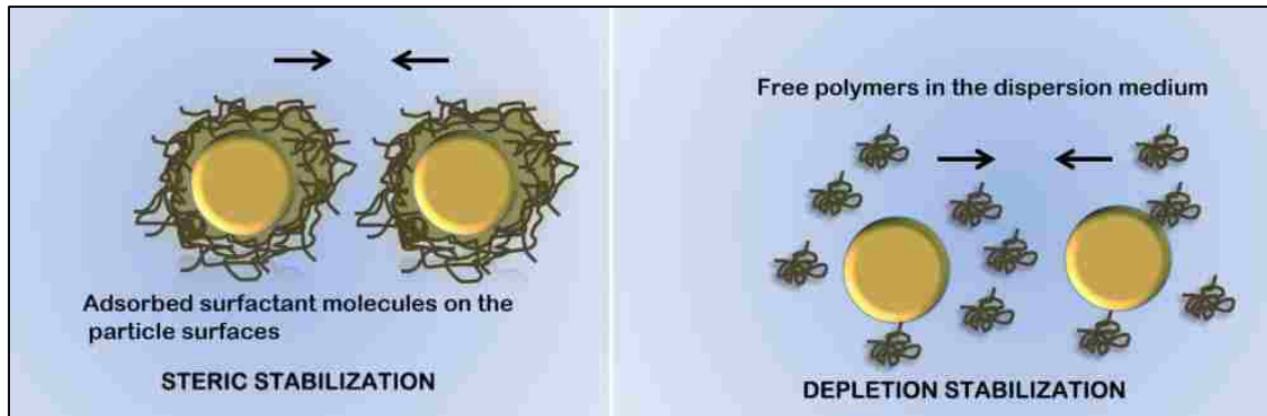
Figure 2-10: Concepts of Steric stabilization (left) and Depletion stabilization (right).
