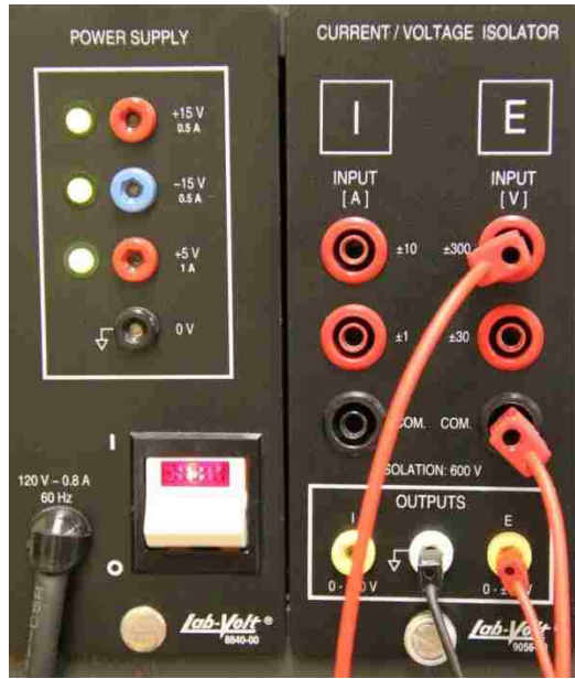
Figure 6.2: Lab Volt’s Current and Voltage Isolators.
