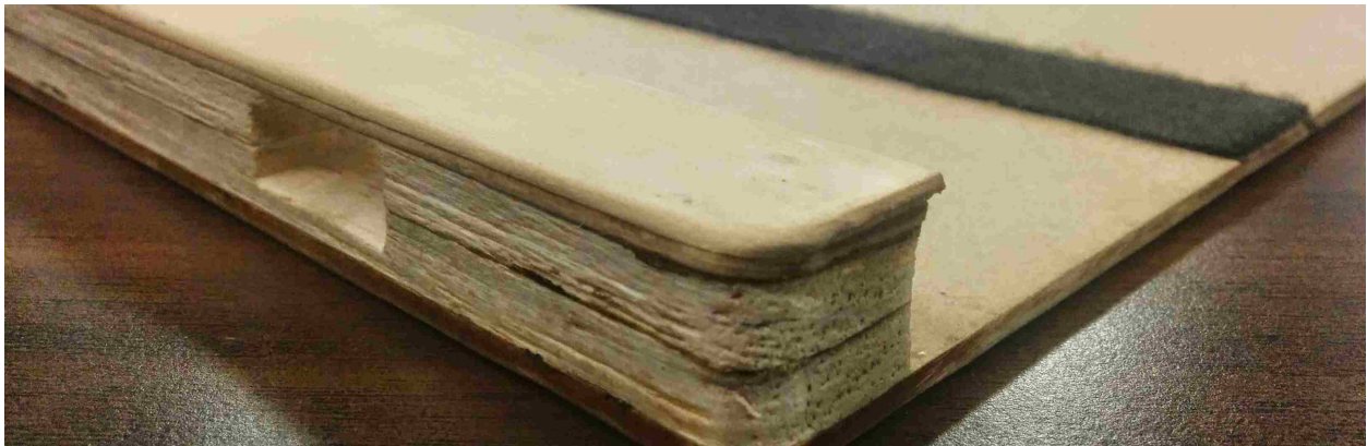
Figure 6.3: Layers in the tablet case
