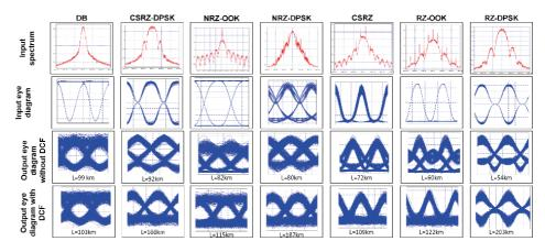
Fig. 3. Input spectra, eye diagrams and output eye diagrams at maximum achievable transmission distance in the systems without and with DCF dispersion compensation module.
