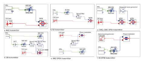
Fig. 2. Different type optical transmitters for implementation of the following modulation formats: (a) NRZ, (b) RZ, (c) CSRZ and CSRZ-DPSK, (d) DB, (e) NRZ-DPSK, and (f) RZ-DPSK.
