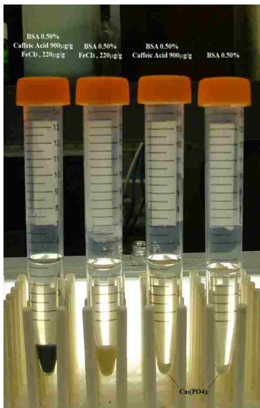
Figure 3.14. Effect of \text{Fe}^{3+} on BSA both with and without caffeic acid, and controls (right).
