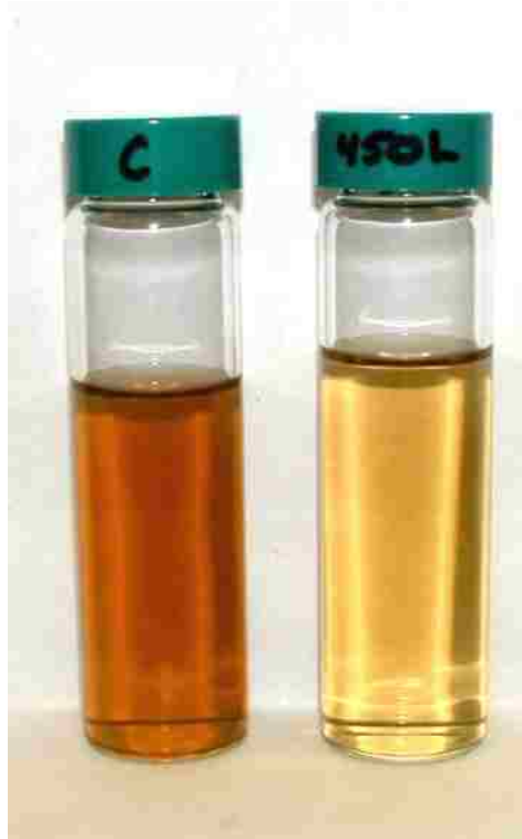
Figure 3.13. Left, raw juice clarified normally via hot liming and right, treated with Fe 3+ the hot-limed.
