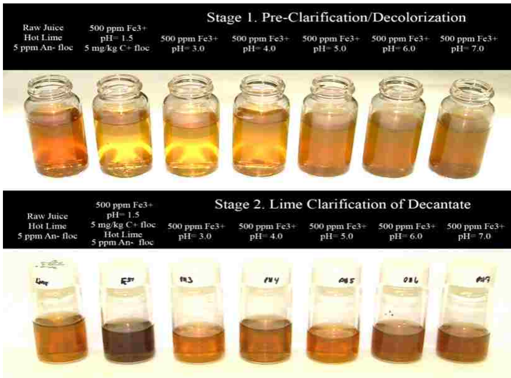
Figure 3.33. The appearance of cane juice clarified hot with \text{Fe}^{3+} (top) and then hot-limed (bottom).
