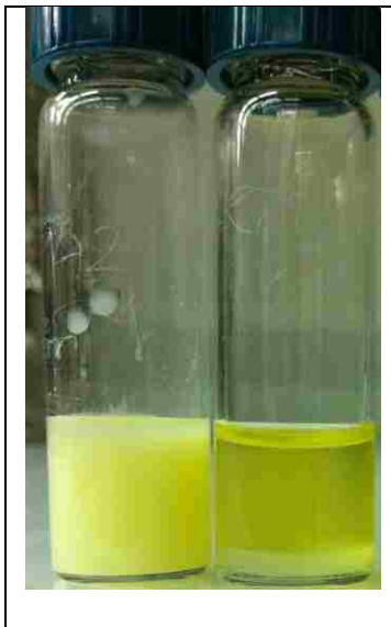
Figure 7.6 Control fluorescent silica cores with no polypeptide loading before (left) and after (right) etching for 40 min. in ~10% NaOH solution.
