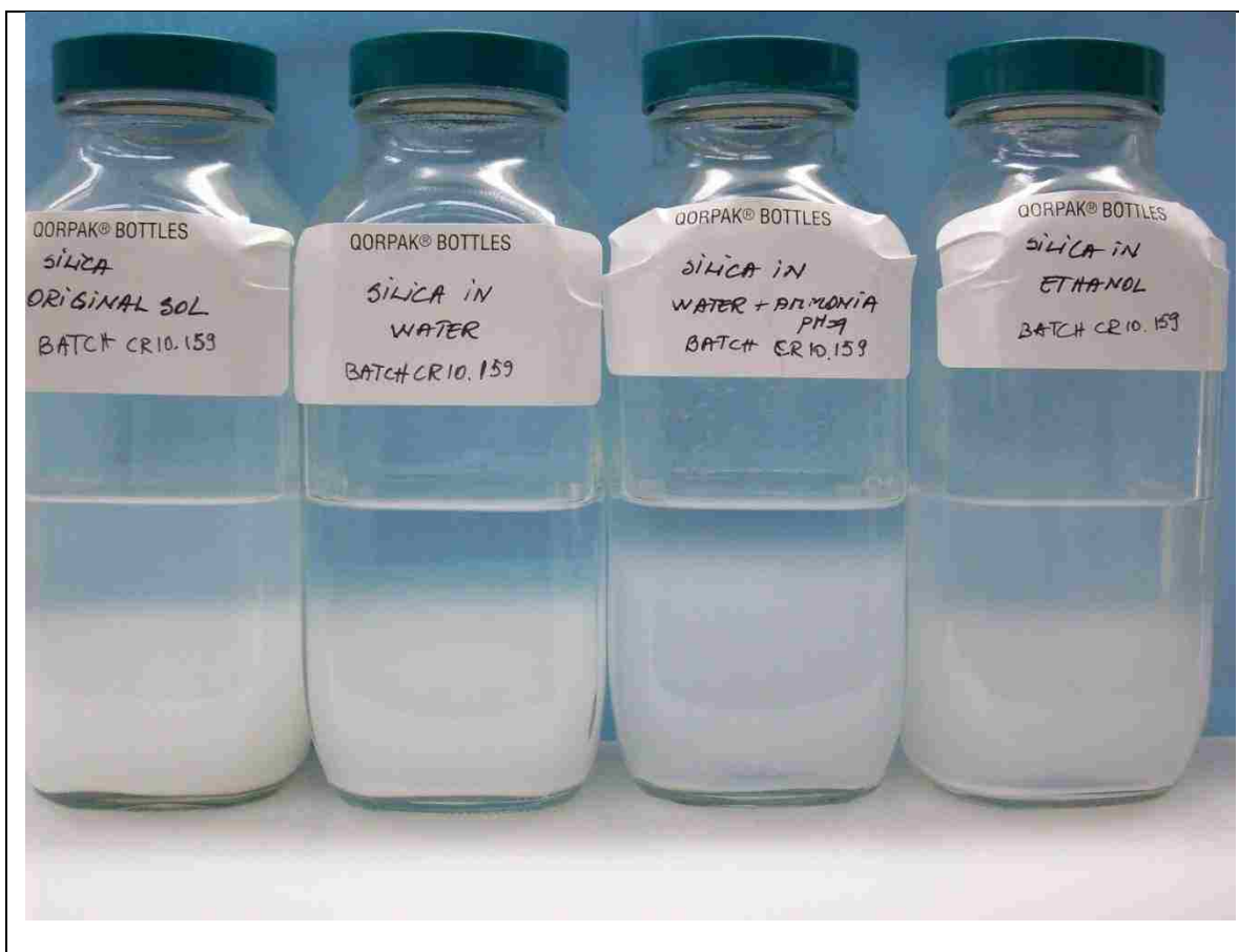
Figure 2.9 Silica seed particles stored in different conditions; from left to right: the original sol, in water, in water and ammonium hydroxide (pH=9) and in ethanol.
