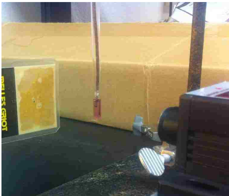
Figure A4.3 Photothermal measurements were recorded by a thermocouple placed about 2 mm above the laser beam.
