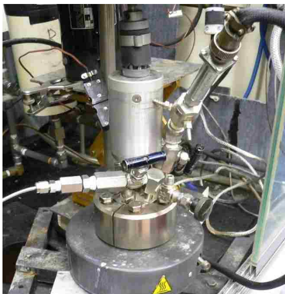
Figure 2.7. Photograph and schematic of previous autoclave design.
