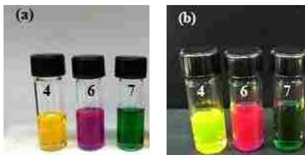
Figure 4.8: Solutions of BODIPYs 4 , 6 and 7 in dilute DMSO under (a) normal and (b) UV light
